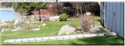
**First** - lay extension ladder flat on its back with feet of the ladder butted up against building's wall and the fly side down.
